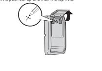
1.7 Remove the door control from the wall and drill a 5/32 inch (4 mm) hole for the top screw.
